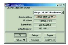
Figure E-2: MAC Address/Adapter Address
